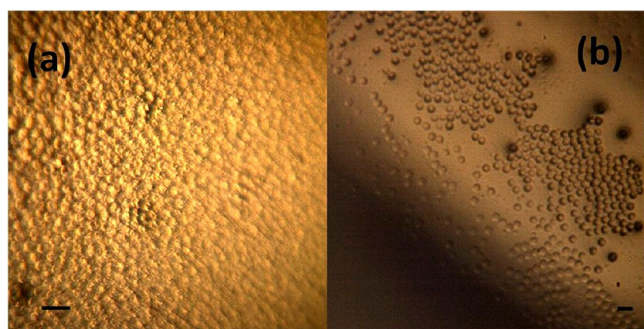
Figure 5. (a) Aqueous silica precursor drops in hexadecane oil phase. Opaueness is observed in the continuous phase near the drops (scale bar 20 \mu\text{m} ). (b) Silica particles in hexadecane oil phase after evaporative processing in collection reservoir (scale bar 15 \mu\text{m} ).
